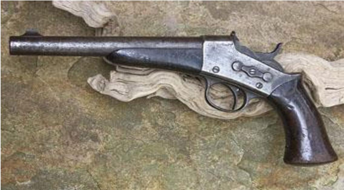
The rolling block mechanism was the inspiration of Joseph Rider who, in May 1864, obtained a patent for a breach loading cartridge gun incorporating an arrangement of the hammer and breach block where the hammer is located behind the breach block and both pivot on independent axis pins. Further refinements were patented over subsequent years.
